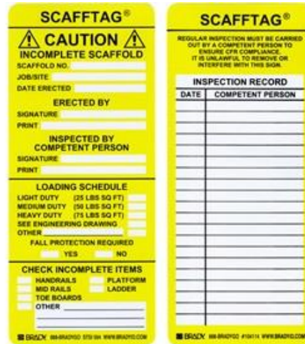
Incomplete but structurally safe scaffold tag (Yellow)
